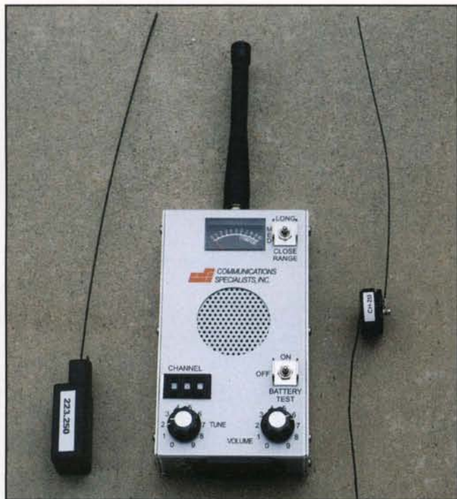
Front view of the R-300 receiver and optional stubby antenna with two miniature transmitters alongside. At left is the 40-mW AT-2B and at right is the 1-mW AT-1B. (Photo by KØOV)
