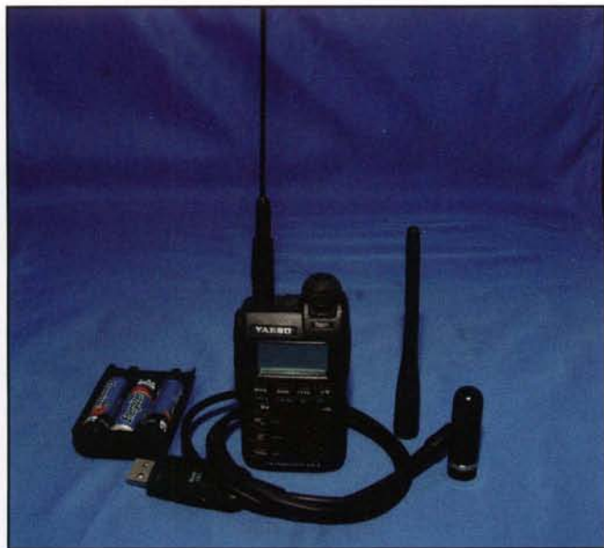
This dual-band miniature HT is a God-send. I picked up two spare antennas—a mini-rubber-duck and a longer dual-band whip (on the HT)—and the stock antenna are shown along with the cloning cable and the spare “AA” alkaline battery pack. This makes up my emergency radio package, which stays with me all the time.
