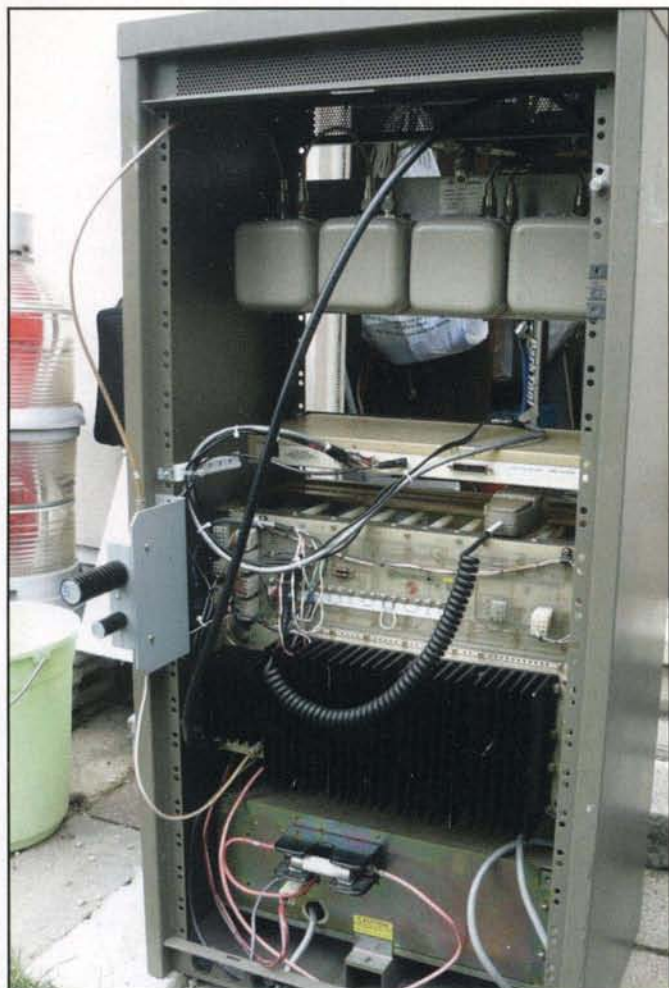
Photo 2. The Rocky Mountain Ham Radio 449.625-MHz repeater uses a GE MASTR II repeater. (Photo courtesy of rmham.org )
