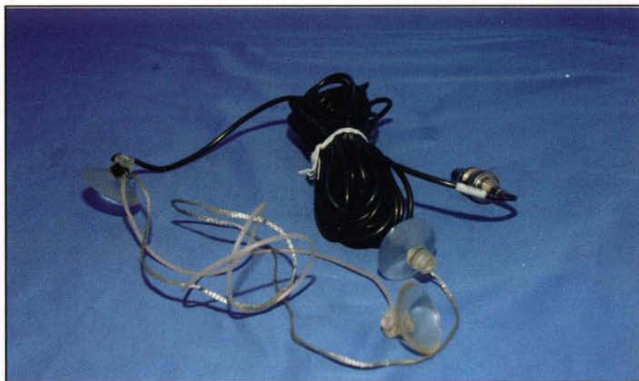
Here is my version of a nifty dipole that originally came with a Bearcat scanner. This one is centered on 146.00 and made from a 20-ft. length of RG-174, terminated in a BNC. This antenna wads up into a very compact and ultra-light package for inclusion in my emergency bag. There is a BNC-to-SMA connector that fits the top of the VX-3R HT. It can be deployed either in vertical or horizontal polarization.
