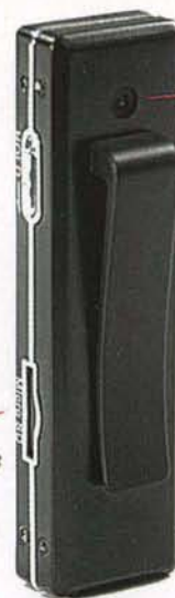
Photo 5. The HobbyPartz mini-FPV video camera weighs less than an ounce.
