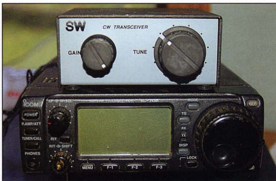
Two of my rigs at home. The ICOM 706 and SW30 are a quick disconnect to put them into the truck or car, whichever is necessary. I carry small, lightweight antennas for HF/VHF/UHF and test them all in the field.
