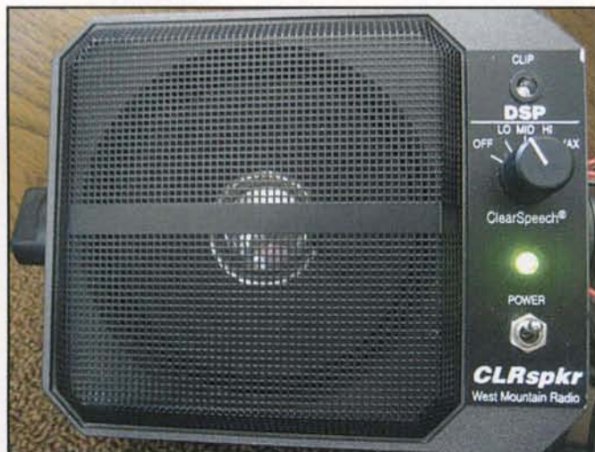
West Mountain DSP speaker, with rotary DSP level adjustment, and green LED showing incoming reception of a signal.
