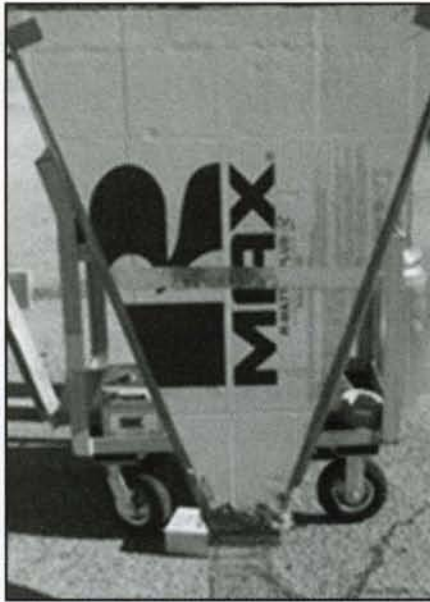
Figures 3 & 4. Inside of foam/aluminum horn with taped seams. Outside of low-cost horn antenna.
