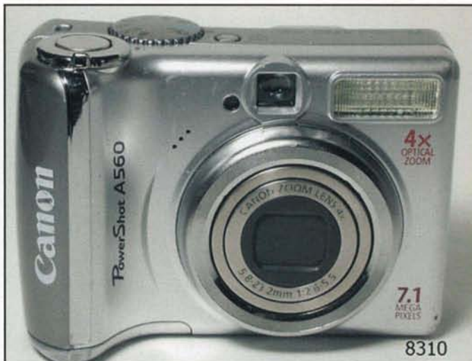
Photo 3. The Canon PowerShot A560 can easily be configured for high-altitude flight with the CHDK script.
