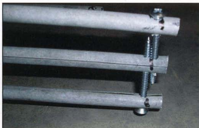
Photo A. Close-up of connecting the elements of the matching system to the driven elements with machine screws.
