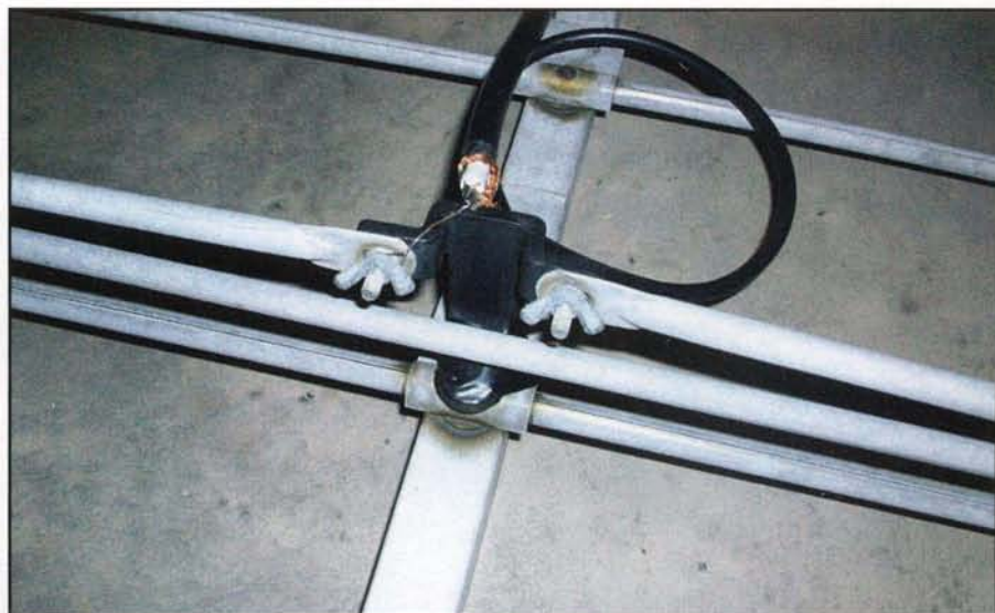
Photo B. Close-up of the coax connection to the folded dipole matching system.
