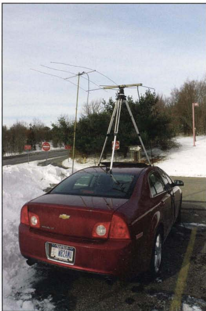
Figure 5. Compared to the various porcupine trucks that have 10-band capability, many hams doing portable or rover operations concentrate on the lower four VHF bands. A new car with a sunroof proved to be very useful for WB2AMU's QRP portable setup on the lower four during the 2011 January VHF contest with the feed lines going from the various antennas through the opening to the radio in the car. (Photo by Ken Neubeck, WB2AMU)
