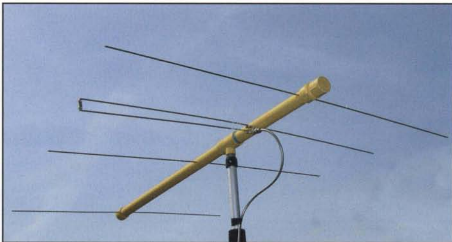
Photo A. The portable "Cheap Yagi" in use. (Photos courtesy of the author)
