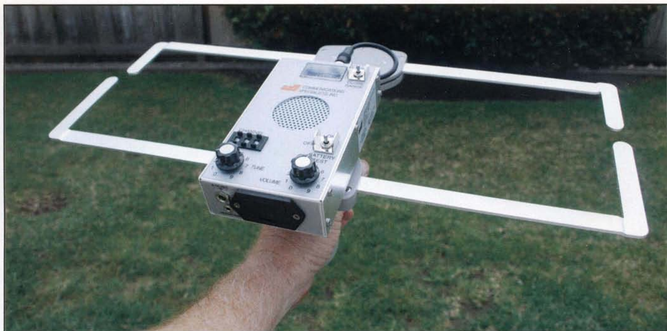
The upgraded R-300 receiver and removable FA-3 Moxon antenna from Communications Specialists. The antenna elements fold in for easy carrying and storage. (Photo by Joe Moell, KØOV)
