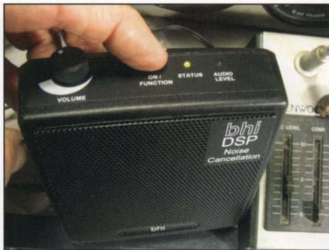
The push-button DSP level adjustment on the bhi speaker.
