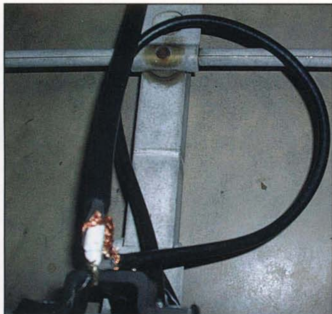
Photo C. Actual balun made from RG-59U.
